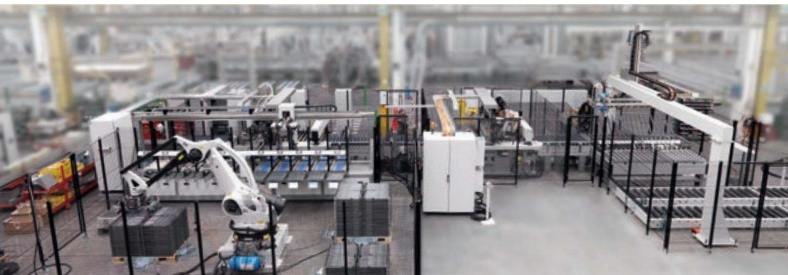
ÉQUIPEMENT FLEXIBLES HAUTEMENT AUTOMATISÉS POUR LA FABRICATION D'ÉLÉMENTS À TIROIRS POUR CUISINES SUR COMMANDE.
